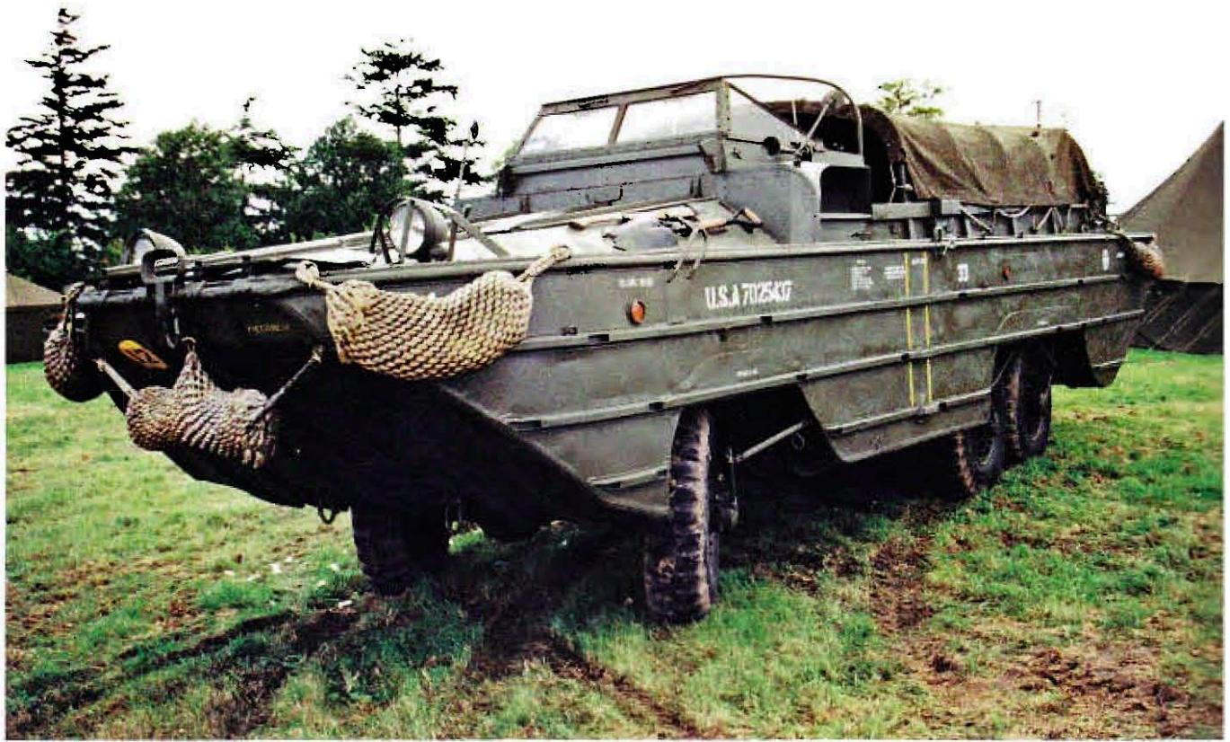
A DUKW (serial no. after DUKW-353-2005), seen in the French camp during the D-Day celebrations, Normandy 1994. The rectangular cutouts in the welded metal rub rails to reduce corrosion are a common sight on DUKWs in postwar service. These cutouts are not featured on dated WW II photos.
